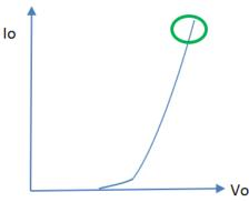
Set V\_overload close to, but higher than the maximum forward voltage for optimized performance. The greater the difference between the V\_overload setting and the maximum forward voltage, the higher the overload stress will be. The V\_overload setting must be higher than Vf.
