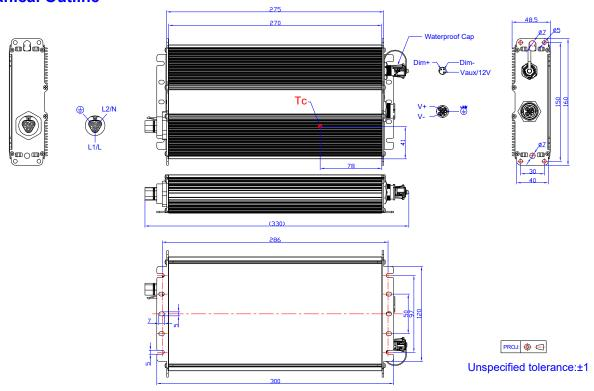
**Note:** This driver features UL Wet Location, IP67 panel mount connectors to streamline wiring in the field while still supporting stringent environmental conditions. The **mating** push-lock are not supplied by Inventronics. Please contact Wieland and Amphenol LTW or one of their suppliers for assistance sourcing the mating push-lock
