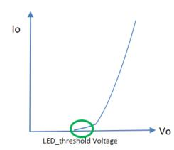
LED threshold voltage (Vth) is the minimum voltage required for current to flow through the LED load. After this threshold is met, the LED forward voltage (Vf) increases as the current increases.
