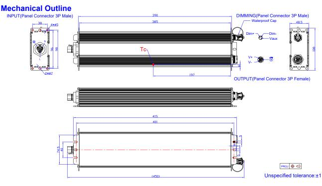
**Note:** This driver features UL Wet Location, IP67 panel mount connectors to streamline wiring in the field while still supporting stringent environmental conditions. The mating push-lock are not supplied by Inventronics. Please contact Wieland and Amphenol LTW or one of their suppliers for assistance sourcing the mating pushlock
