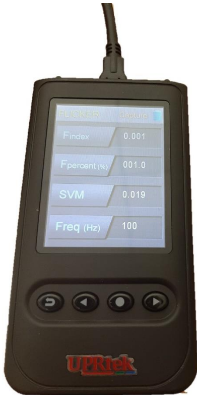
Image 4: Inventronics' EUD-480S140DV readings from a handheld spectral flicker meter.
